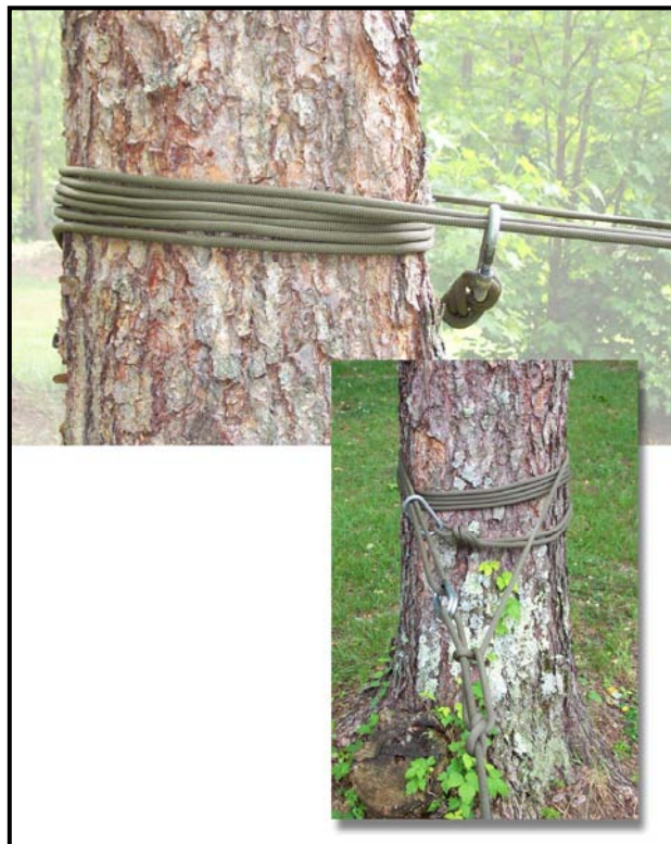
Figure 7-13. Tensionless anchor knot.
